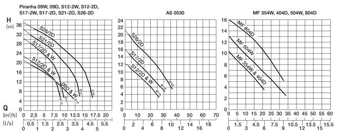
H = Total Head; Q = Discharge Volume. Curves to ISO 9906 (60 Hz available on request) N.B. please use the ABSEL program to validate pump selection.
