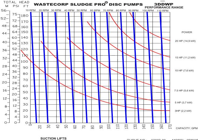
Dry Prime Static Suction Lift: 25' (7.62m) Wet Prime: 25" Hg 28.4' (8.6m)
