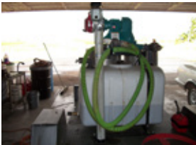
Waste oil skid mounted pump
