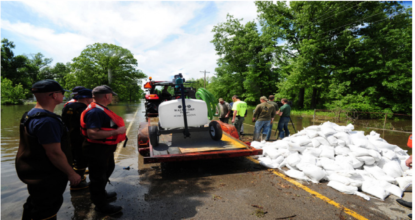
HW-150-ATV Series portable waste recovery system. 150 gallon tank, ATV hitch for towing with (John Deere Gator, Kawasaki Mule, Polaris, Volunteer, Bobcat, etc). Three way valve system for pumping both into and out of the tank. Installation used by the National Guard to contain an oil spill from an industrial facility during a flood.
