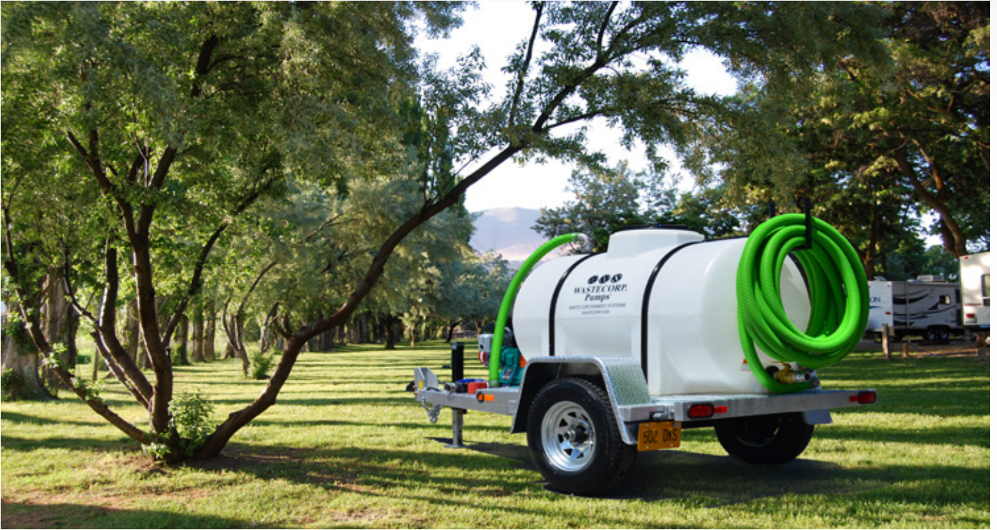
HW-300-DT Series honey wagon waste containment system. Galvanized deck and frame, engine driven Mud Sucker pump technology. 325 gallon tank with DOT package (electric brakes and lighting package). This installation used to pump out RV black water tanks, portable toilets and septic waste.
