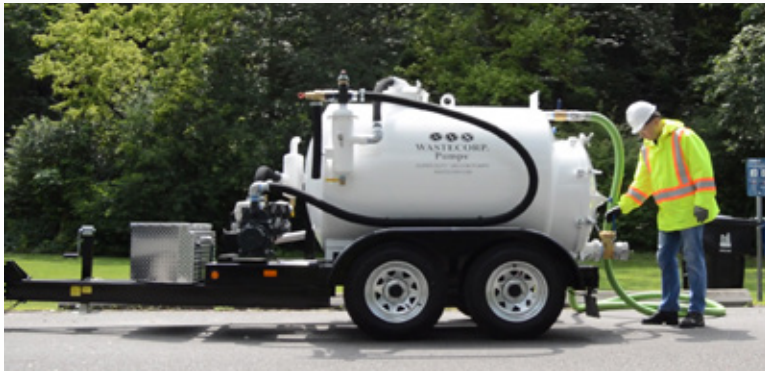
TVP-450, 450 gallon model shown with DOT compliant trailer and optional storage bin.
