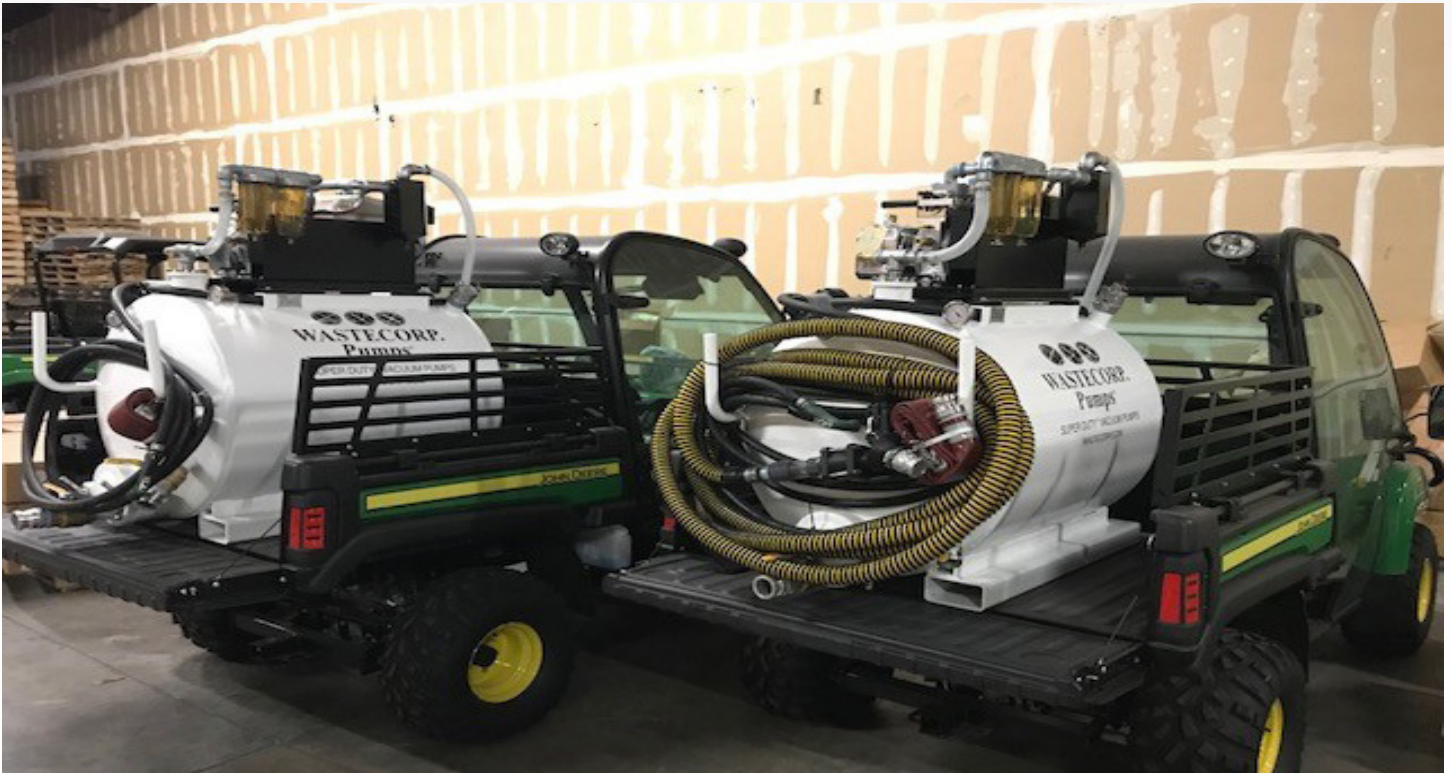
Super Duty TVP-150 Series, 150 gallon vacuum pump systems mounted in the rear bed of John Deere Gator utility vehicles. Top mounted vacuum pump to conserve space, alternate pump mountings available. Designed for high suction power around government operated sports/entertainment complex. Ideal for facilities maintenance, septic, waste oil and grease.
